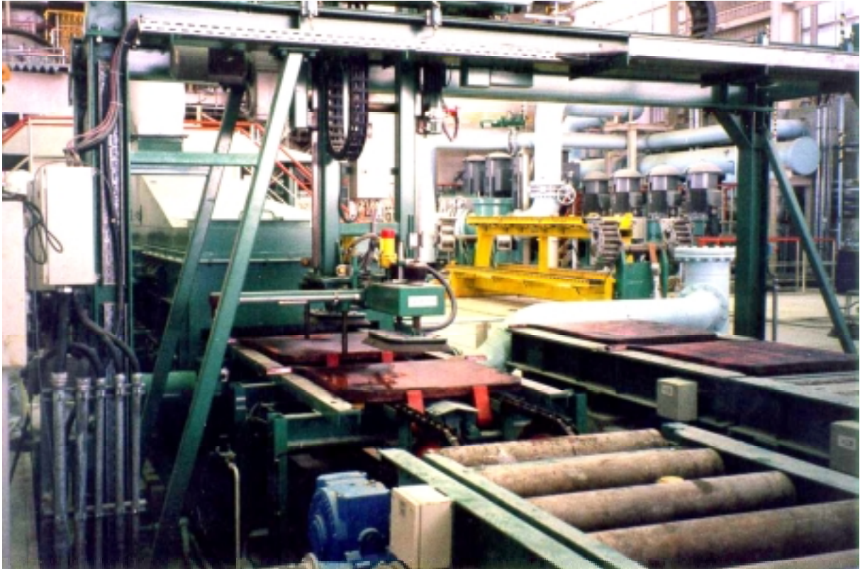
Figure 12: Cooling tunnel, transport conveyor chain and stacking device
